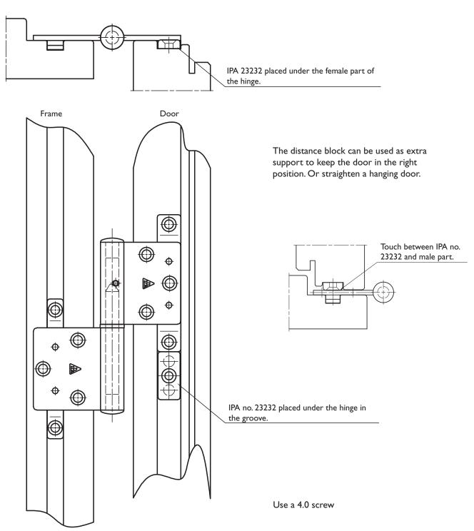
The distance block is used in IPA system fitting, for example IPA no. 11198.
